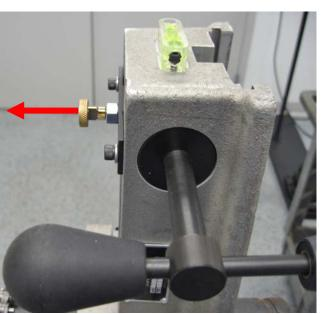
Pull Part Number 276899 retractable spring plunger out and turn 90 degrees. This allows the feed handle to turn freely.
