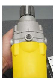
Threaded hole where lower block will be attached.
