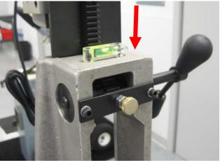
Place Part Number 701063 plate (with drill attached) into the slot of frame. Turn Part Number 276899 retractable spring plunger knob 90 degrees to lock feed handle.
