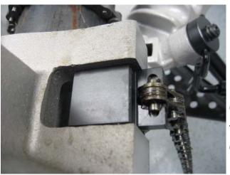
Once chain is hooked into the block, turn Part Number 606742 Handle in the clockwise direction to tighten frame to pipe.
