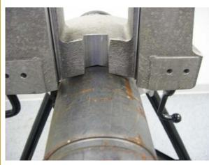
Make sure the machined "V" in the bottom of the frame is centered on the pipe.
