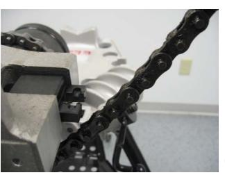
Pull the chain upward and place into the Part Number 700993 chain hook block. (see below)
