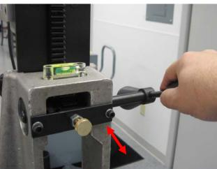
Once the drill has been placed into the frame, hold the feed handle and pull the retractable spring plunger knob 90 degrees to unlock feed handle before and after drilling.
