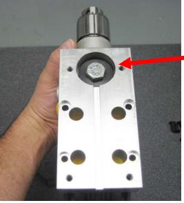
Assemble Hex Screw and Mounting Plug in drill body. Do not tighten.
