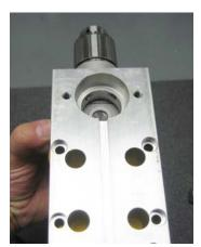
Place lower block on drill with counterbored hole facing up.
